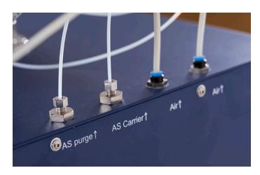
Helium is used as a carrier gas to transport the resulting gases from the combustion reactor through various filters to the TCD. The system consists of an auto-sampler (AS), a combustion reactor (CR), a reduction reactor (RR), three water traps (F1, F2 and F3) and a carbon dioxide adsorber (F4), and the thermal conductivity detector (TCD).
